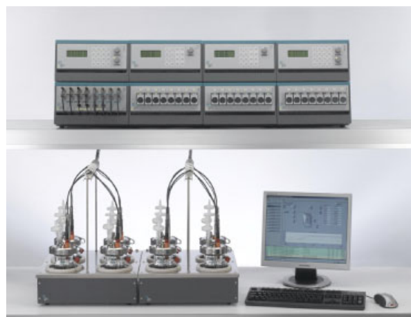
Figure 3. The whole biofuel development procedure can be represented on a small scale by integrating the multi-step processes into one bench top bioreactor system (Source: DASGIP AG).
